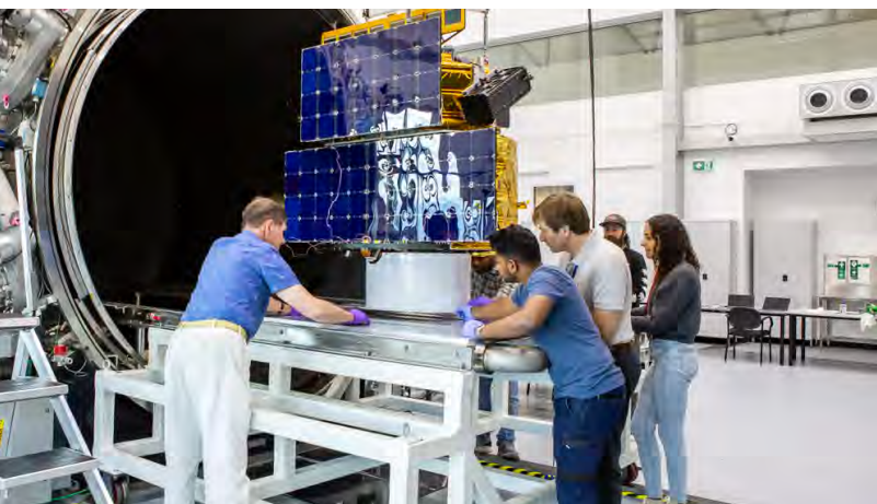
NSTF Team and Space Machines Company Team preparing the Optimus Platform spacecraft for the experimental activities in space conditions in the Wombat XL (Photo credit: Cristy Roberts, ANU)
