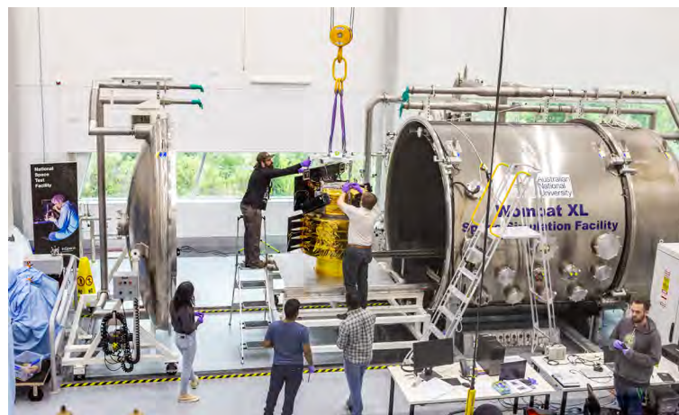
NSTF Team and Space Machines Company Team preparing the Optimus Platform spacecraft for the experimental activities in space conditions in the Wombat XL (Photo credit: Cristy Roberts, ANU)
